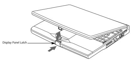
Figure 3-2 Opening the Display Panel
